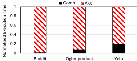
Fig. 2: Normalized Execution time of SpMM and GEMM matrix operators in a single representative forward propagation layer of a multi-layer GNN model.
