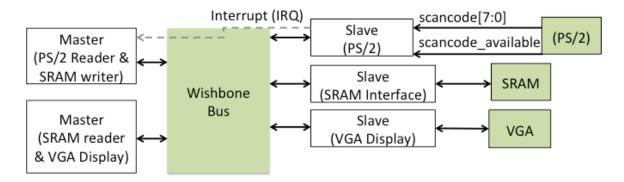
The VGA controller with a Wishbone interface is provided to you. The SRAM interface is the same as from lab5 and the PS/2 Keyboard interface is the same as from lab6.
