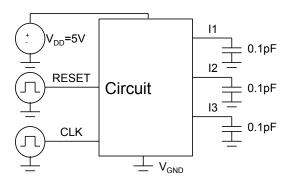
The simulation setup is shown above. The only parts that are to be used internal to the circuit are NMOS and PMOS transistors from the AMI05LIB. Your simulation should go for 6 clock cycles. In the first and last clock cycles, the RESET line will be high. In all the other clock cycles it will be low.
