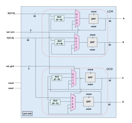
You will enter the VHDL designs for the ALU and DFF modules and port map four instances of each in the pa1.vhd. The 2-bit select signals are used to control the four 4:1 multiplexors, and they are derived using the computed four 32-bit outputs, A, B, C and D.
